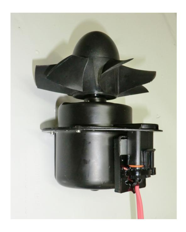
Regulator is carefully plugged into the Generator body as seen Above. Press in place using the the back end of the module plug until latch clip is properly seated. Do not force! If there is any issue, check the alignment of the tangs of the plug exiting the GenniPod body.
