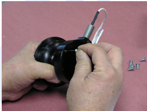
Figure 3.1: Installation of MTH Alignment Pin on an EA-3000 MTH
