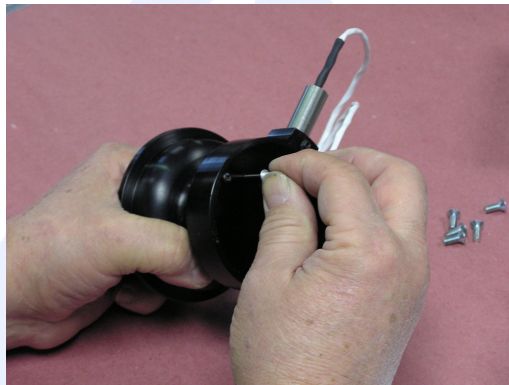
Figure 3.1: Installation of MTH Alignment Pin
