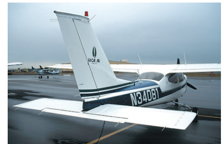
Figure 1-7 Vertical stabilizer and rudder.
