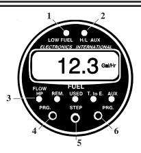
Blinking "REM" LED on Power-up: After power-up, the FP-5(L) will blink the Fuel Remaining (REM) LED and display the fuel remaining in the tank(s). The "REM" LED will continue to blink until any button or switch is pushed. The blinking "REM" LED is intended as a reminder to update the FP-5(L) if you've added fuel to the aircraft since the last flight.
